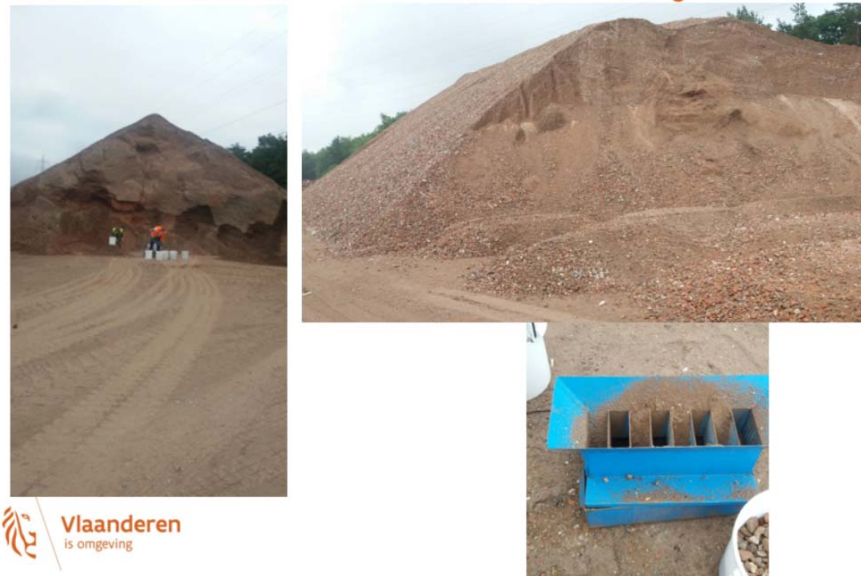
Fig.6: Sampling of asbestos from recycled construction waste.
