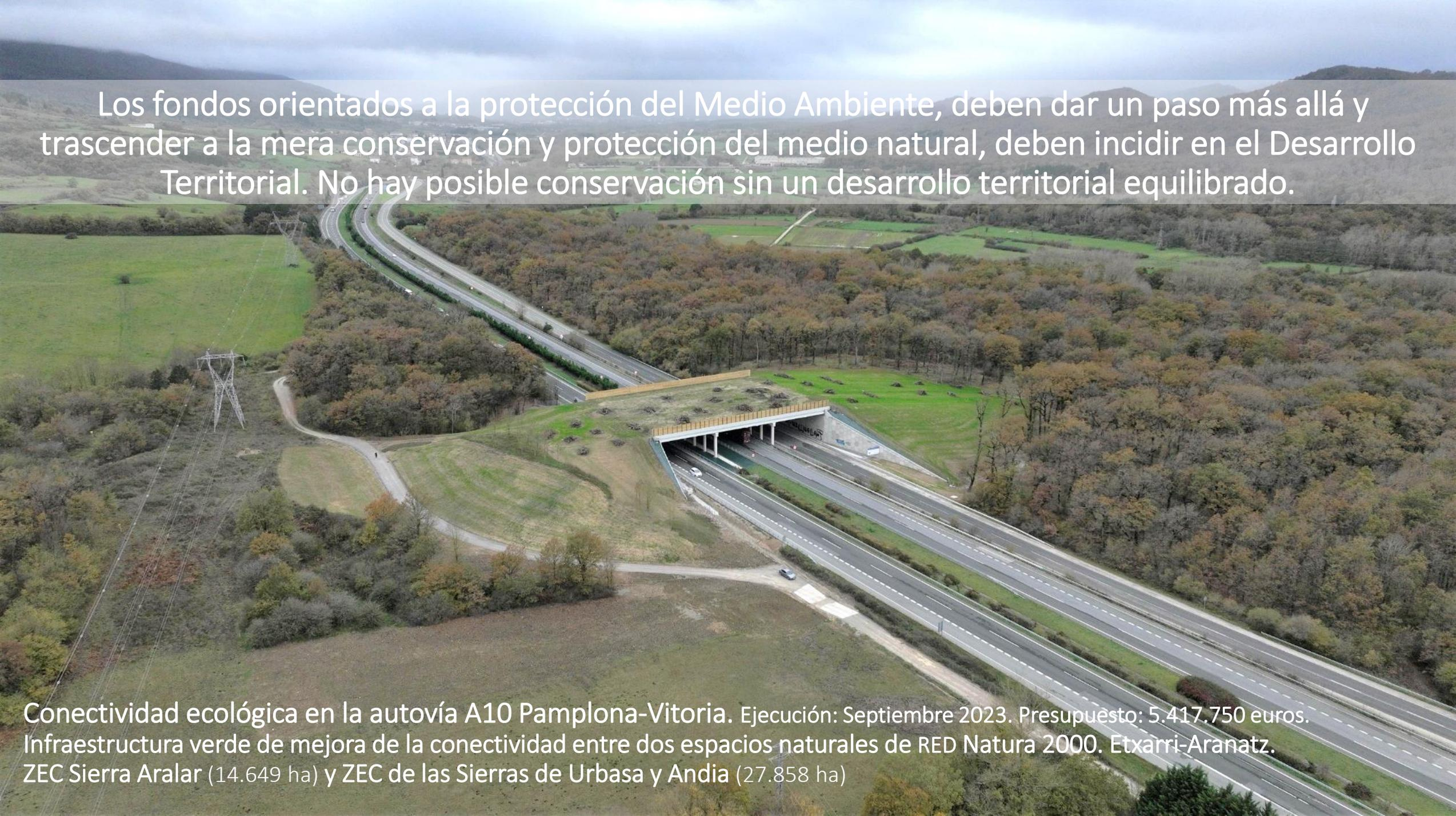
An aerial photograph showing a multi-lane highway (A10) passing through a landscape of green fields and dense forests. A prominent feature is a large, green-roofed bridge or overpass structure that spans across the highway, designed to maintain ecological connectivity. The bridge has a flat roof covered in grass and small plants, supported by concrete pillars. The surrounding area includes a dirt path, a utility pole, and rolling hills in the background under a cloudy sky.
